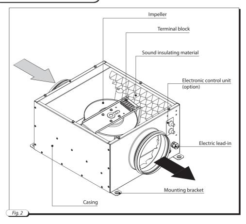
The fan casing is made of galvanized steel sheets internally lined with heat- and sound-insulation layer. The round spigots are rubber sealed for airtight connection to the air ducts, Fig. 2.
