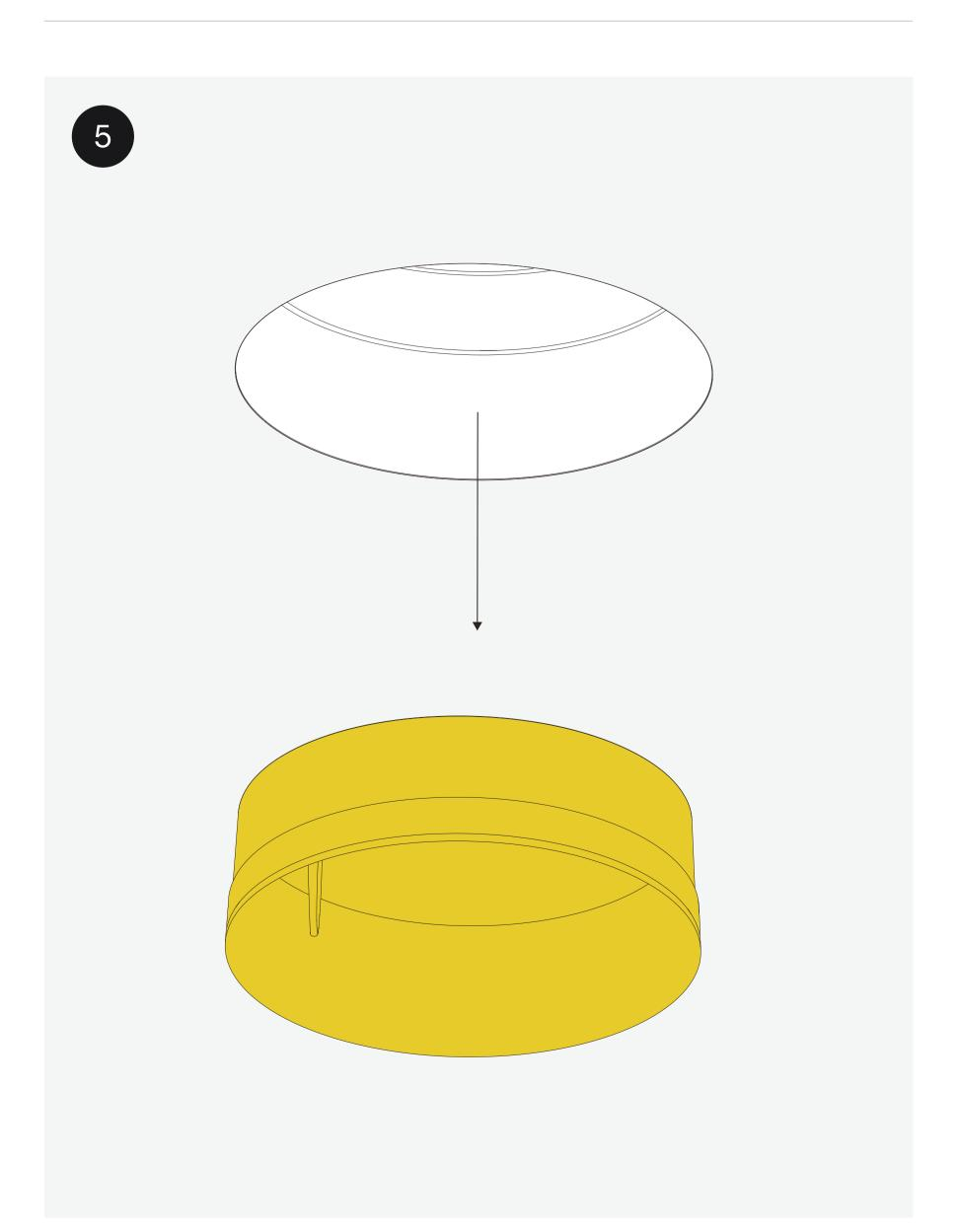
Remove the plaster lid just before installing the fixture. It helps to keep the inside of your plaster ring free of filler, paint and dust. Any residue needs to be removed without damaging the edges of the plaster ring. thank you for choosing prado
