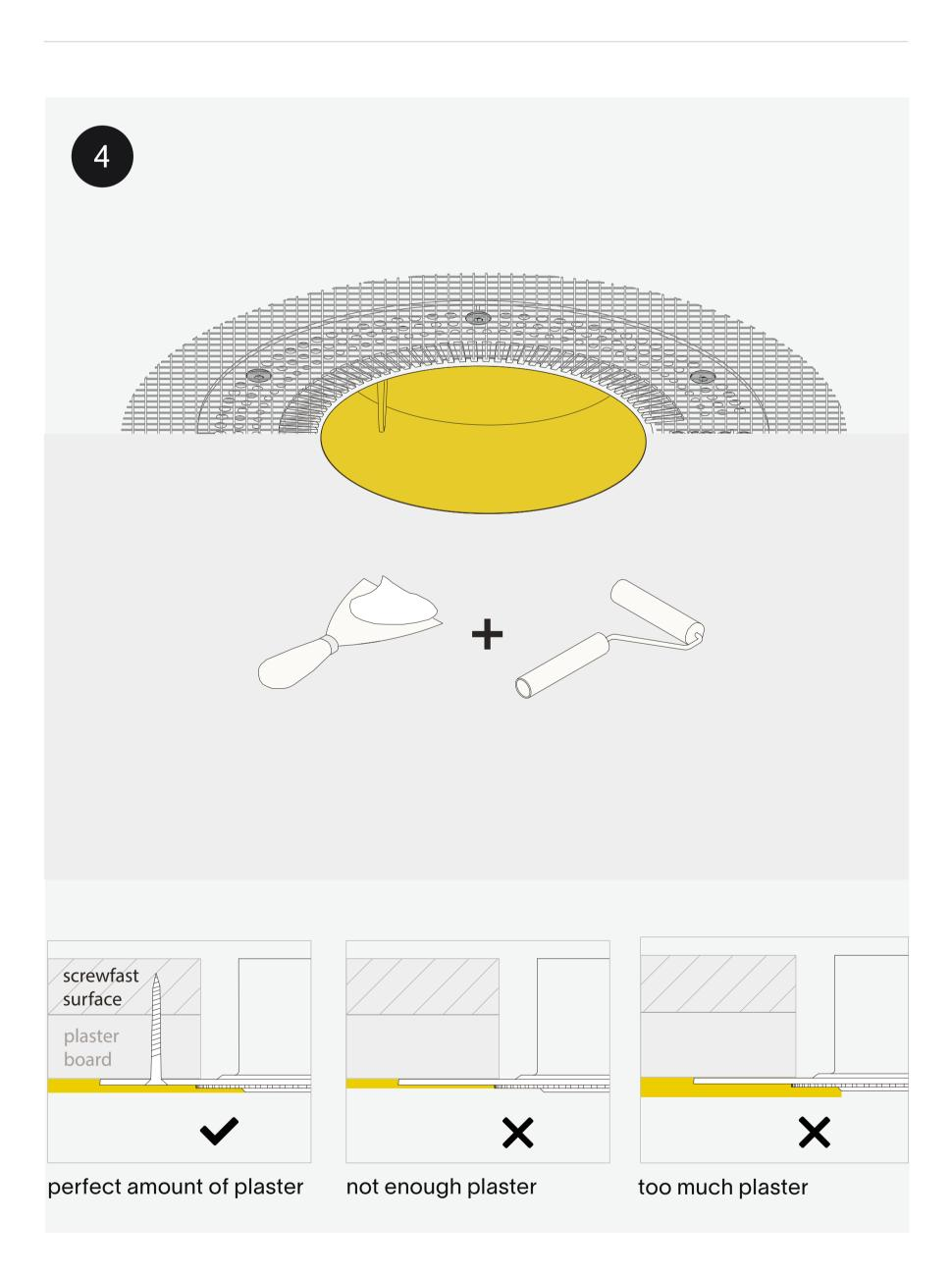
Excercise caution while plasering, do not damage the ring. Keep the plaster lid inside the plaster ring while
