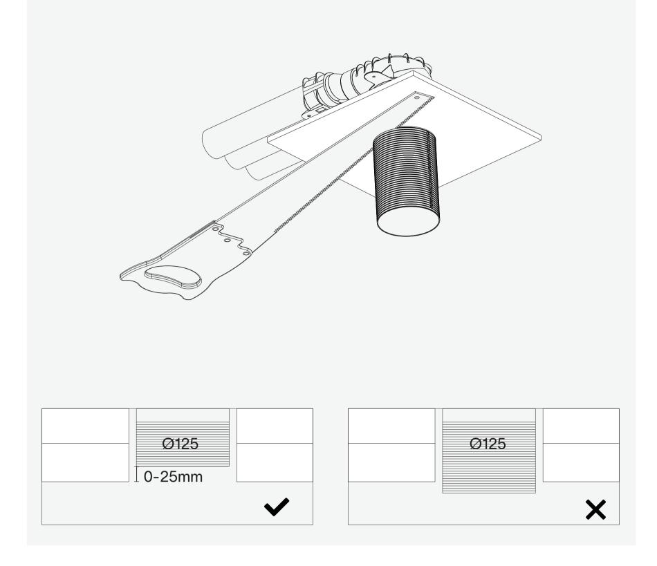
Cut off the excess length of the valve adapter. (between 0 and 25 mm above final ceiling level) The remaining vertical part of the adapter (before the start of the turn) must be at least 75 mm high for the plaster ring.
