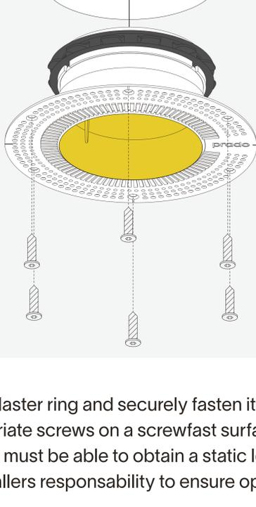
Insert the plaster ring and securely fasten it with glue or the appropriate screws on a screwfast surface. The attachment must be able to obtain a static load of 5 kg. It's the installers responsibility to ensure optimal attachment.
