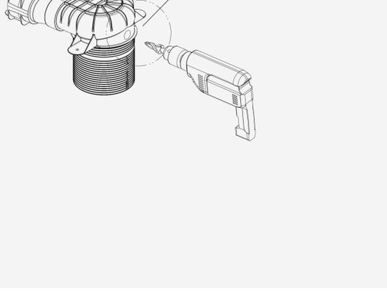
Use a step drill to cut a Ø20 hole into the Ø125 valve adapter of your choice. A hole can be drilled in any type or brand of Ø125 valve adapter.
