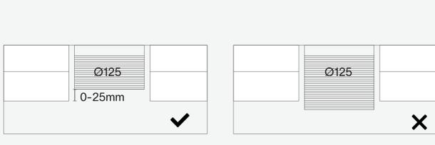
Cut off the excess length of the valve adapter. (between 0 and 25 mm above final ceiling level) The remaining vertical part of the adapter (before the start of the turn) must be at least 75 mm high for the plaster ring (connector can't be placed in this zone).
