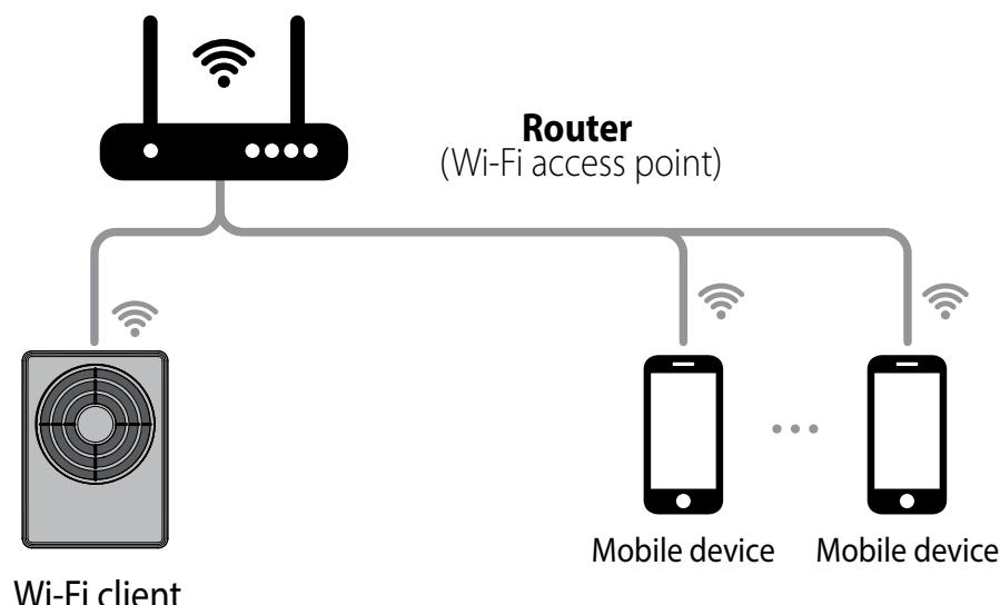
**Example 3:** BMS Smart Home system connection via router with several Wi-Fi access points.
