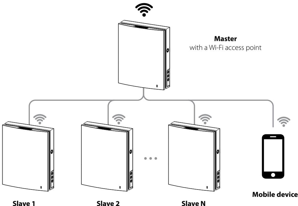
2. Master devices, slave devices, mobile devices and a „Smart Home“ system connect to the Wi-Fi access point of the network router. In this case the maximum number of available Wi-Fi connections is limited by the router functionality. If the number of necessary ventilation units is more than the router can accept, you may use an additional Wi-Fi access point to connect the remaining ventilation units. The router network may include several master devices to provide control by zones.
