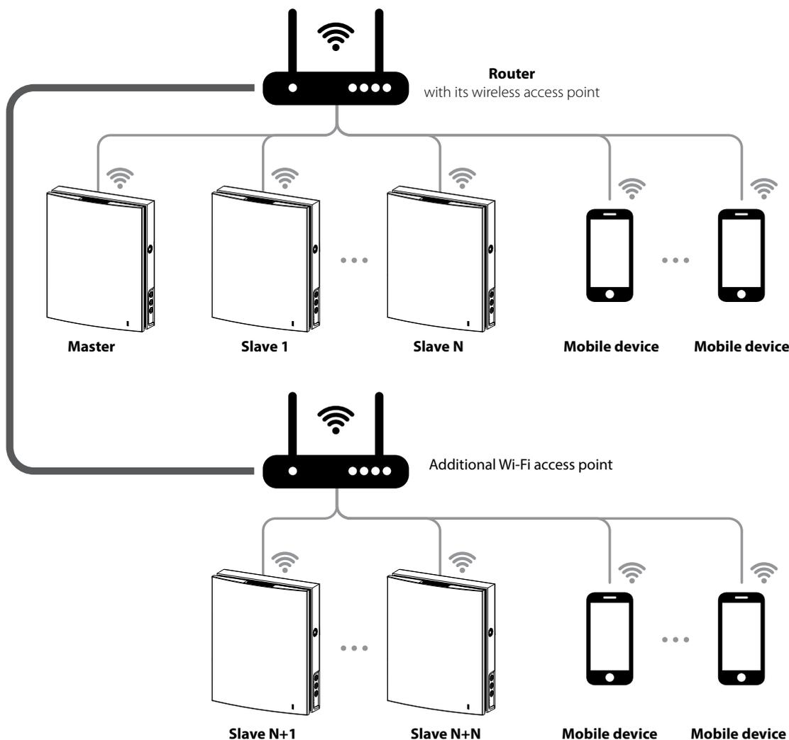
The connection is set up via the mobile application from the Connection –> Wi-Fi setup menu (see the unit data sheet).
